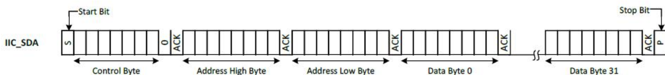
Figure 6-3 I2C page write format
