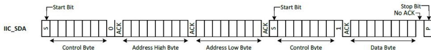
Figure 6-5 I2C random read format
