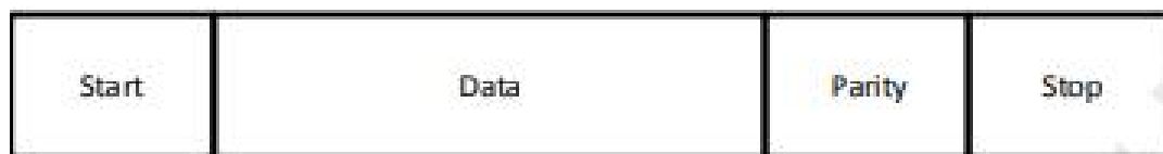
Figure 6-12 UART Data Frame
